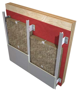
Cross laminated timber with cladding
