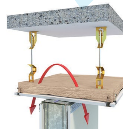
Figure B4: Sound Transfer Over Partition
