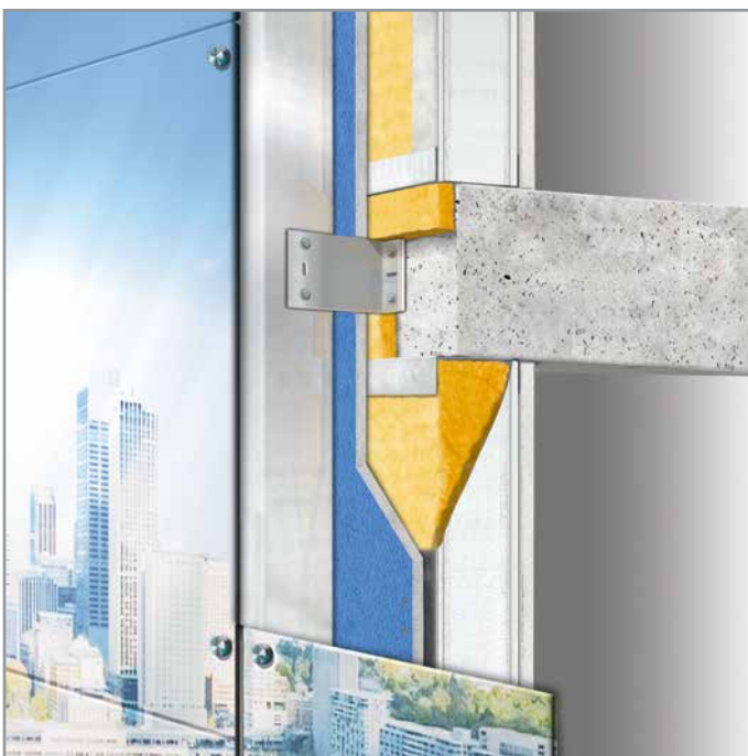
Ventilated Façade with glass cladding
