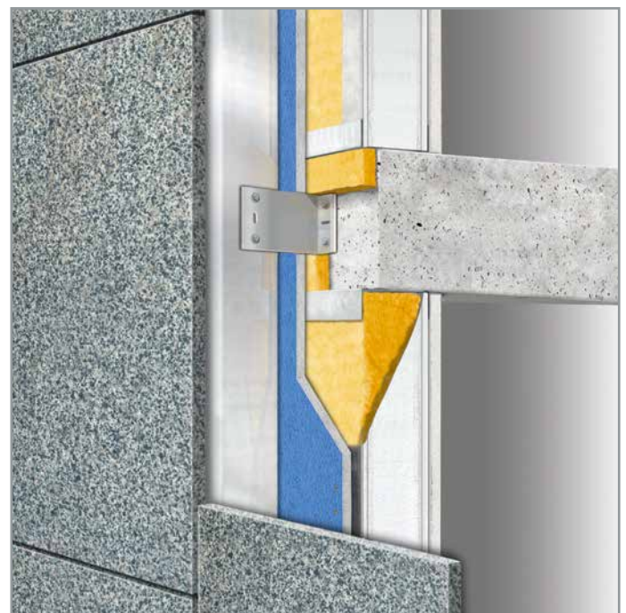
Ventilated Façade with stone cladding
