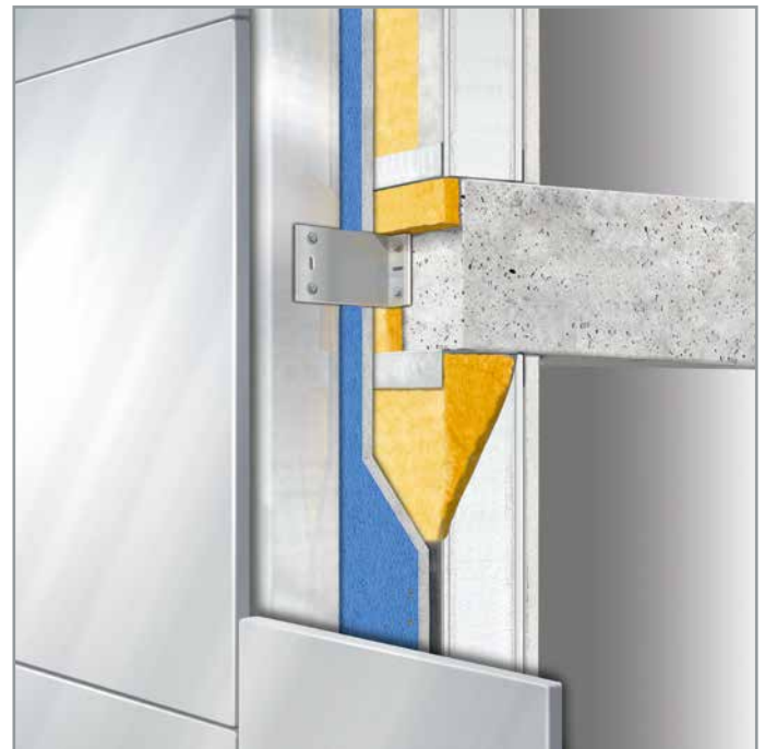
Ventilated Façade with aluminium cladding
