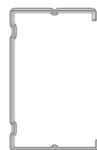
Metal Structure of Profile 1 x CW 100/0.6
