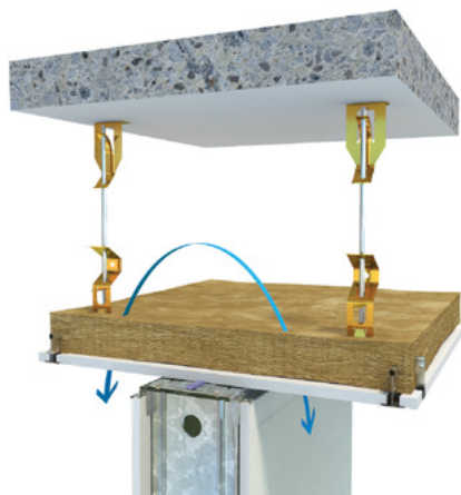
Figure A5: Sound Transfer Over Partition
