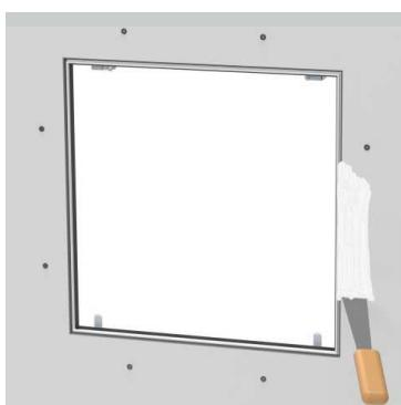
EN - Fill the mounting frame and the flap lid separately using a joint filler. Clean the metallic interior and side surfaces of the mounting frame and the door leaf after further coating of putty and paint residues!
