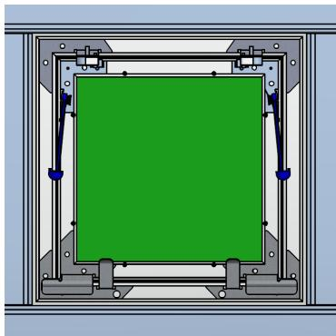
EN - Install the support profile CD with a gap of 5 mm at each side between the mounting frame.
