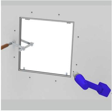
EN - Screw the mounting frame and fit the screws with the protective caps that are supplied along. (It is recommended to attach the lid to ensure proper mounting before next step).
