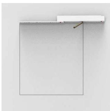
EN - Mark the structural dimension and cut an opening into the wall (approx. 3-5 mm larger than the nominal dimensions). 100mm void needed if mounted from front.
