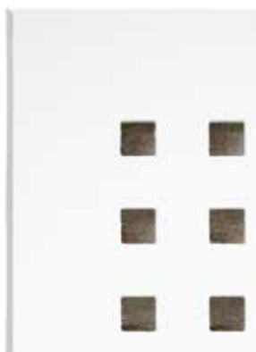
Quadril, 12 x 12 mm, 30 mm c/c Perforering: 13%
