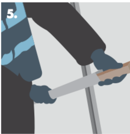
5. Insert timber battens within Knauf 'C' Studs to provide fixing for door frame (if required).
