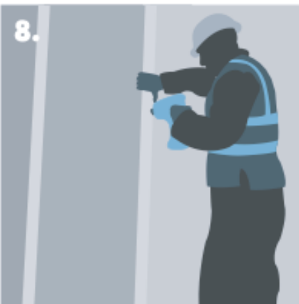
8. Fixing Knauf Plasterboard to the completed framework.
