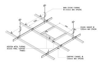
Recommended Access Panel Ceiling Frames (600mm x 600mm)
