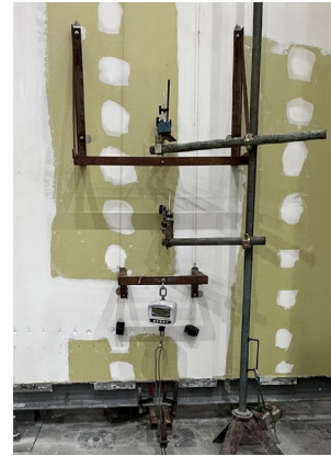
Figure 30: Heavy weight anchorage (downward loading - wash basin)
