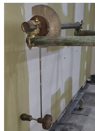
Figure 23: Perforation by small hard body
