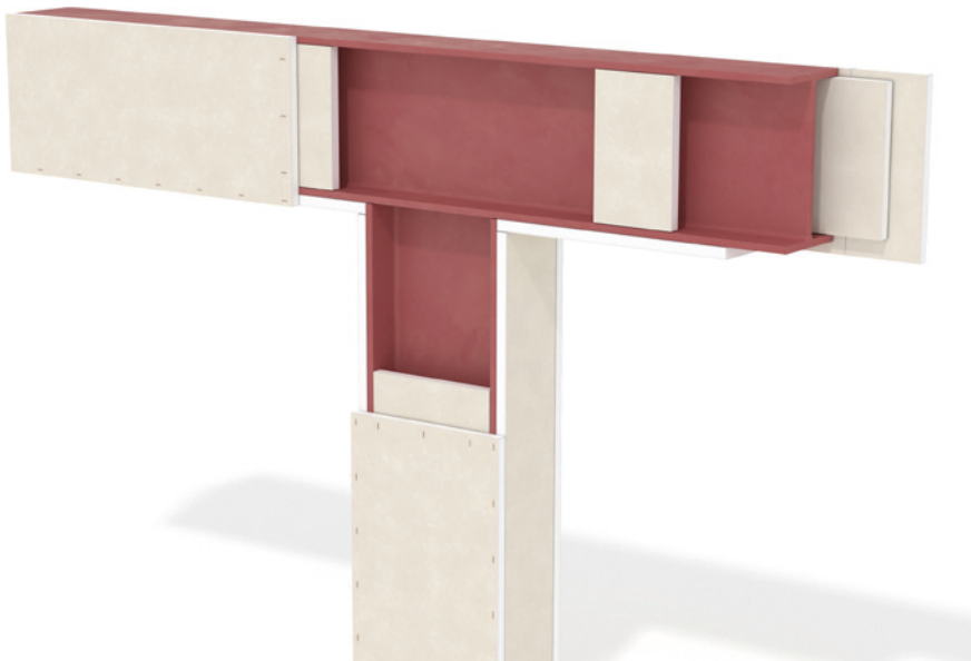
Figure 1: Representation of Knauf Fireboard Frameless Encasement System
