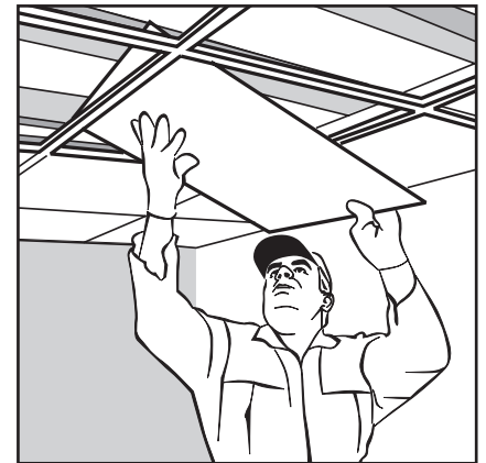
4. Placing the tiles in the grid frames
