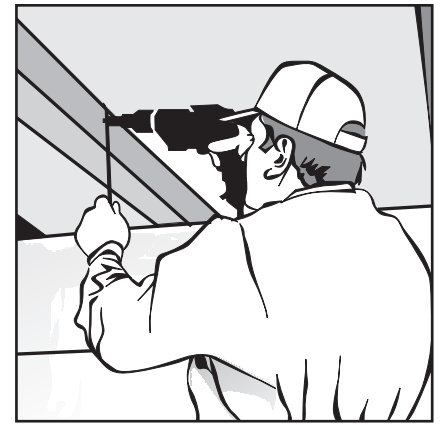
2. Fixing the hangers to the main soffit
