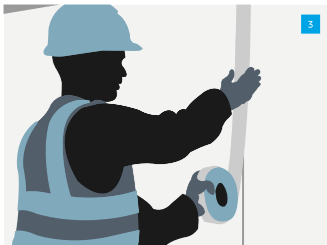
Taping the joints with Knauf Windliner Tape.
