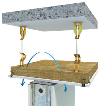
Figure A5: Sound Transfer Over Partition
