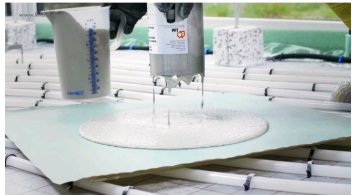
Image 3: Lift the consistence checking tin
