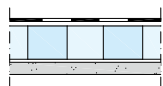
12.5 mm Cleaneo Klett Board with foil lamination on the rear side and Cleaneo Klett Surface
