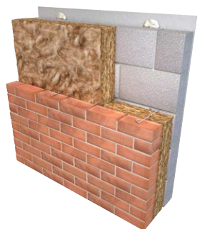
External Masonry Cavity Walls - Fully filled
