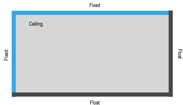
Figure 2: Perimeter fixing on adjacent edges
